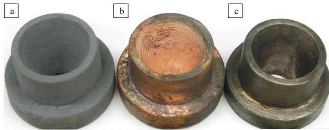
Figure 2. Demonstration of net-shape/size DCP processing (of rocket nozzles). a) Porous, rigid WC nozzle preform prepared by 3-D printing, then binder burnout and light sintering (to neck WC particles to enhance preform rigidity). b), c) ZrC/W nozzles formed by immersing the porous WC preform in Zr_2Cu(l) at 1150^\circ C , then reaction above the melt at 1300^\circ C . Adherent Cu-rich metal on the surface of the specimen in b) (pushed out from inside the specimen during the pore-filling DCP reaction) was removed from the specimen in c). d) Measured dimensions are shown of a reactively-converted nozzle in c), and of the associated porous WC preform prior to infiltration (dimensional changes were \leq 0.85\% ).
