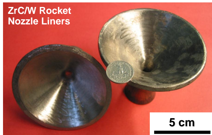
Figure 3. ZrC/W rocket nozzle liners fabricated by: a) gel-casting to generate a porous WC nozzle liner, b) immersion of the porous WC nozzle liner in molten Zr_2Cu at 1200^\circ C for 10 min, and c) completion of the DCP reaction upon heating to 1300^\circ C to yield dense, near net-shape and near net-size ZrC/W nozzle liners. Such liners placed within a carbon composite backing material yield lightweight nozzles resistant to the extreme thermal shock and erosion of a solid-fuel Pi-K rocket test.
